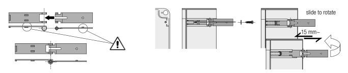
Snap the cover onto the hinges. Close it and secure it using the supplied screws. After the settings and adjustments, fasten the cover using the supplied screws.
