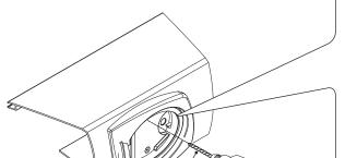
Hole for the left-hand motor release rod
