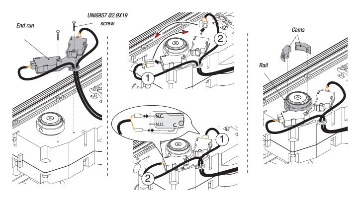
Close the leaf fully and turn the cam clockwise until the closing microswitch is activated. Secure the cam with the screws.
