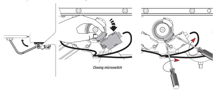
Fully open the leaf and turn the other cam anti-clockwise until the opening microswitch is activated. Secure the cam with the screws.
