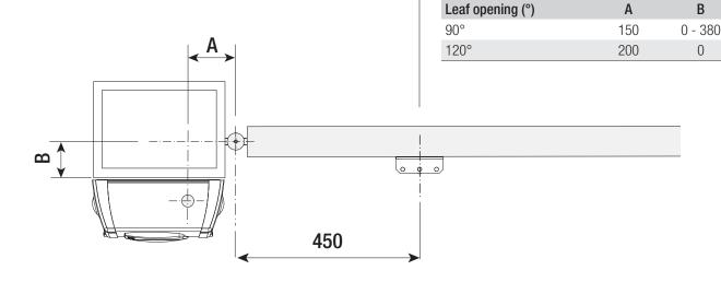
Mark the fixing points on the pillar bracket and gate bracket, respecting the values shown in the drawing.
