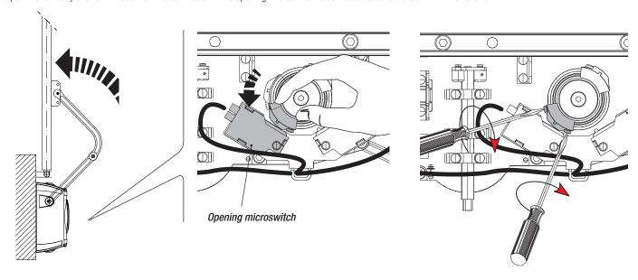
Close the leaf fully and turn the other cam clockwise until the closing microswitch is activated. Secure the cam with the screws.
