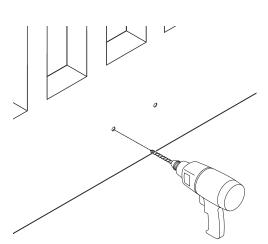
Insert the anchors or use suitable inserts for holding the brackets.
