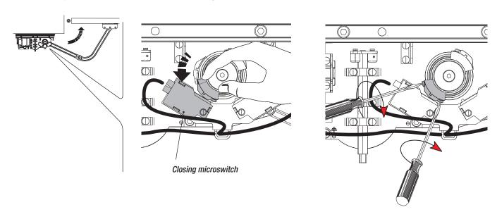
Fully open the leaf and turn the other cam clockwise until the opening microswitch is activated. Secure the cam with the screws.
