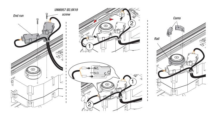
Open the leaf fully and turn the cam clockwise until the opening microswitch is activated. Secure the cam with the screws.
