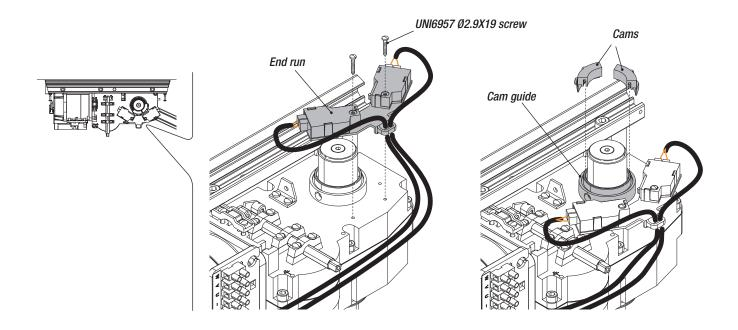
Open the leaf fully and turn the cam anti-clockwise until the opening microswitch is activated. Secure the cam with the screws.
