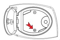
Connect the earth wire to the motor. Put on the cover.
