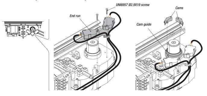
Close the leaf fully and turn the cam anti-clockwise until the closing microswitch is activated. Secure the cam with the screws.
