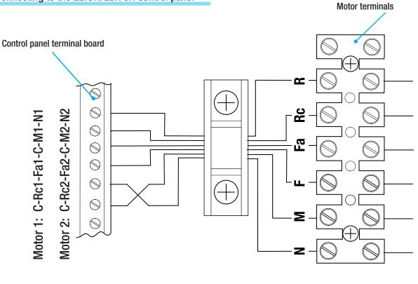
M -N Connecting the motor F -Fa Opening endstop microswitch
