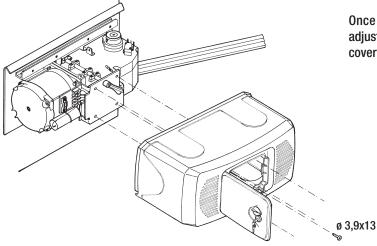
Once finished with mounting, electrical connections and adjustments, lock the motor back into place and replace the cover securing it with the 4 issued screws.
