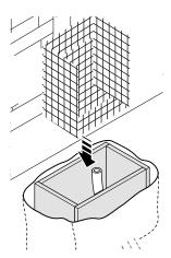
Fasten the anchoring clamps to the plate by using the supplied screws, washers and nuts. Fit the anchoring plate into the iron cage.
