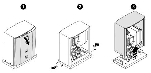
Place the operator on top of the anchoring plate.
