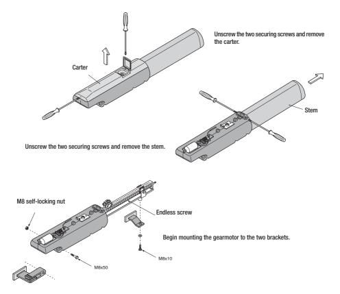
N.B.: we suggest lubricating (using neutral grease) the endless screw and the bushing upon installation.
