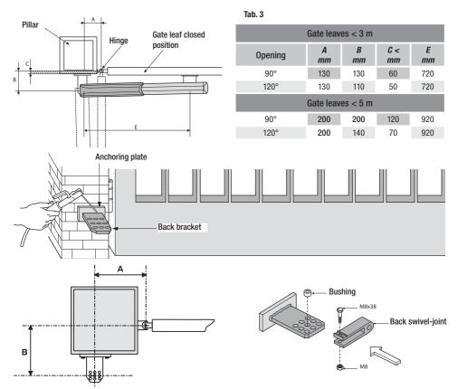
Apply the anchoring plate to the pillar using the back bracket (fig. 1) making sure the A and B measurements are right (Tab. 3) between the hinge axis and central bore hole on the bracket. The back bracket has several other holes for changing the opening angle of the gate.
