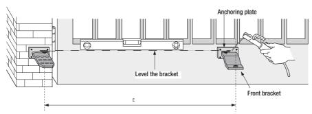
With the gate closed apply the anchoring plate to the gate leaf, making sure that the front bracket is lined up horizontally with the back bracket and ensuring that measurement E is met.
