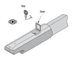
Release the gearmotor and swing the gate-leaf to the fully open position you desire, then, unscrew the securing screws on the opening stop micro-switches assembly.
