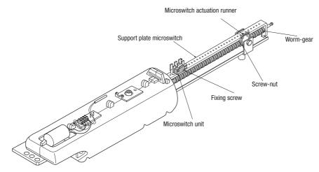
Release the gearmotor and move the door to the maximum desired open position. Loosen the fixing screws of the microswitch unit
