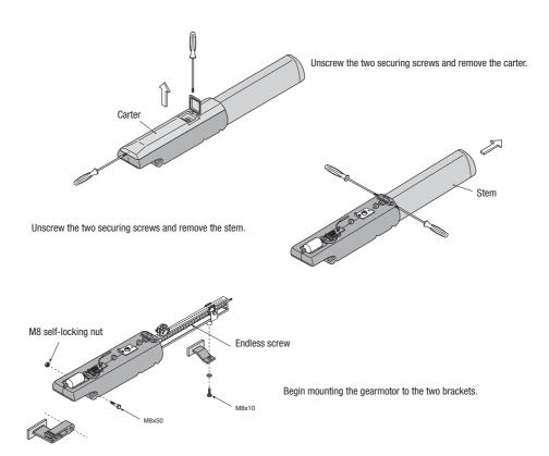
N.B.: we suggest lubricating (using neutral grease) the endless screw and the bushing upon installation.
