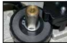
Mechanical twin-disc bath clutch
