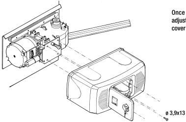
Once finished with mounting, electrical connections and adjustments, lock the motor back into place and replace the cover securing it with the 4 issued screws.
